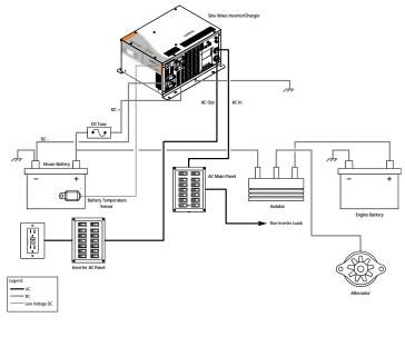
Figure 2 Sample Vehicle Electrical System Configuration
